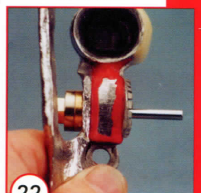
18 Replace the housing into metal base
